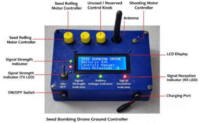
Fig. 7. Control system integration
