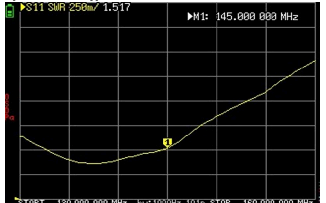
Fig. 10. VSWR of Assembled Eggbeater Antenna
