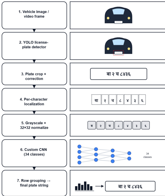
Figure 3: Multi-stage Nepali ANPR pipeline.
